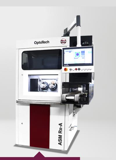
The OptoTech 4-axis generator ASM Rx-A is the ideal universal automatic grinding machine for ophthalmic mineral lenses. Spheres, aspheres, torical, A-torical up to free form surfaces can be produced in highest precision and accuracy. The machine offers high quality grinding due to 2 interpolating axes.
