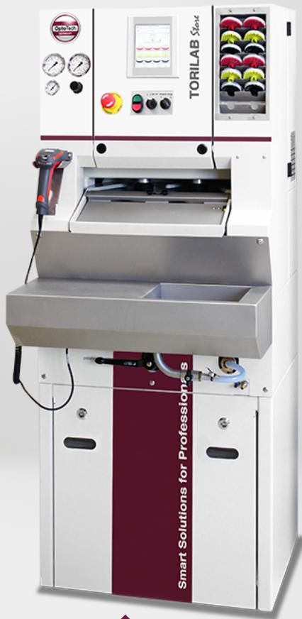
The OptoTech Torilab Store is a 2 spindle machine for polishing toric, spheric and freeform design lenses with only a handful of OptoTech new developed flex tools. The tools have an excellent tool life time so the consumable cost for operating a Torilab Store will be extraordinary low.
