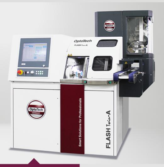
The new digital surfacing-turning machine FLASH Twin-A is an enhancement of our tried and tested FLASH series. Due to the usage of 2 Fast Tools, the FLASH Twin-A is able to simultaneously process 2 freeform lenses. Considerably increased speed of the tool spindles, combined with a high-class precision ball bearing, leads to significant improvements in quality and quantity. It is the ideal complement to our ESM Twin-A.
