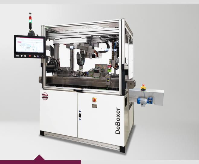
The new automatic DeBoxer is the first ever fully automatic system to specifically unpack semi-finished lenses. Depending on the type of boxes, this machine can unpack up to 300 lenses/h. Moreover, the DeBoxer can optionally be equipped with 2 outgoing conveyors for direct waste separation in carton and plastic.
