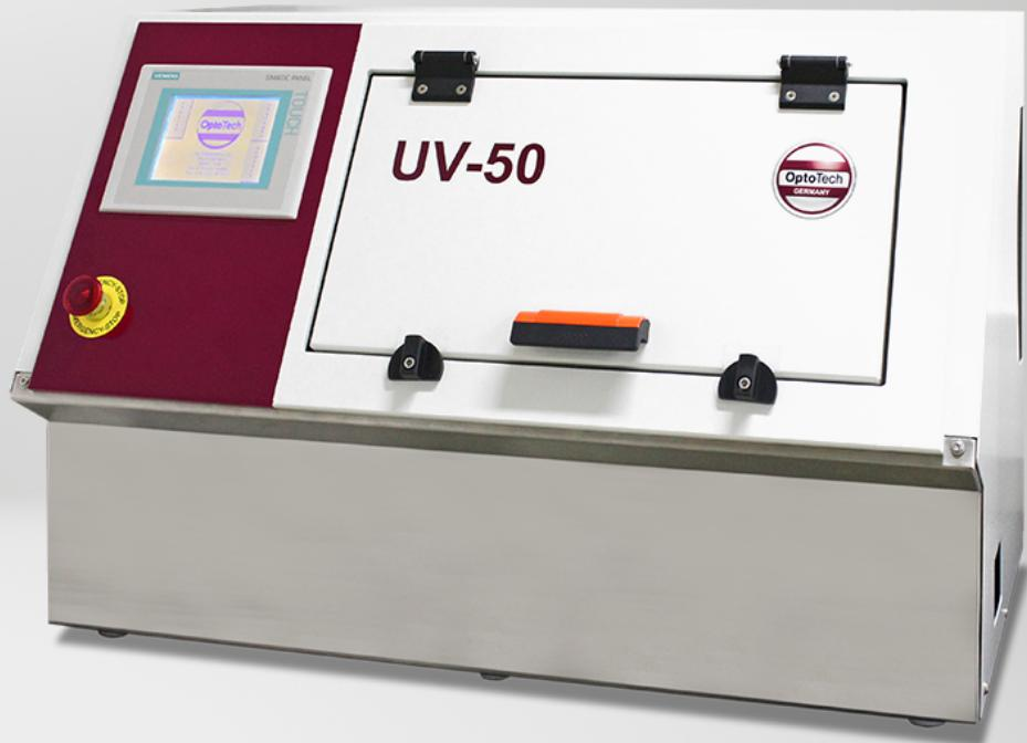
Quality test of the coating through accelerated aging under treatment with heat, humidity and UV-radiation.
