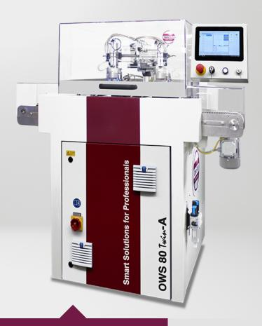
The OWS 80 Twin-A was especially developed for automatic cleaning and drying of blocked or unblocked (option) ophthalmic lenses on a very small footprint. This machine is equipped with 2 cleaning and drying stations, allowing the OWS 80 Twin-A to clean and dry at least 240 lenses/h.
